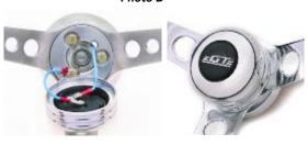
Reconnect battery and test operation of horn and turn signal canceling.
